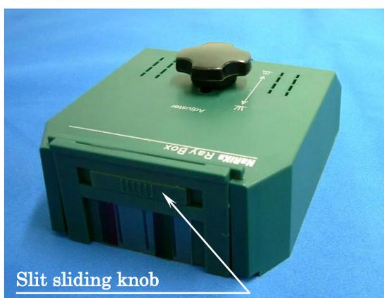
Photo 3 Front Panel of Light Source Unit
