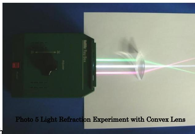
Photo 5 Light Refraction Experiment with Convex Lens
