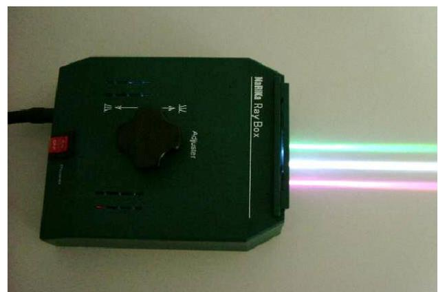
Photo 4 Three Optical Path Outputs through Slit Plate
