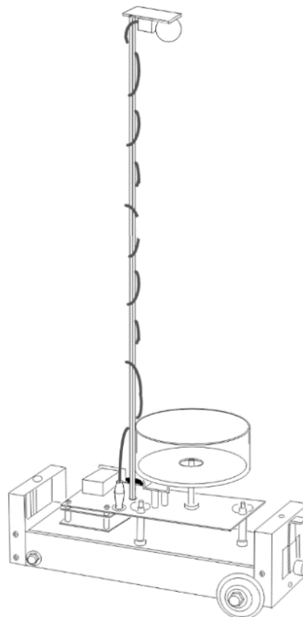
Fig. 6 Completed free-fall device
