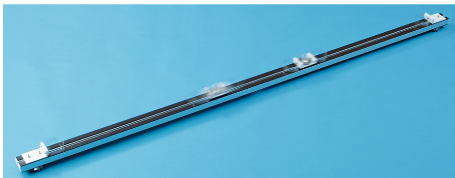
Fig. 1 Sliding body traveling test on magnetic floating track
