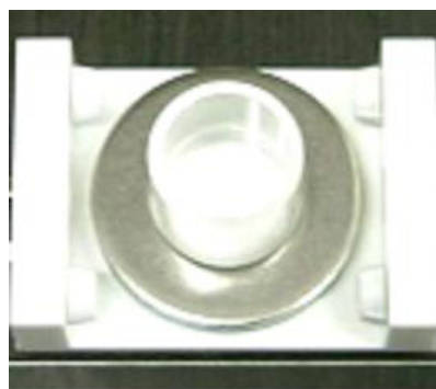
Attach the supplied weight plate to the acrylic pipe
