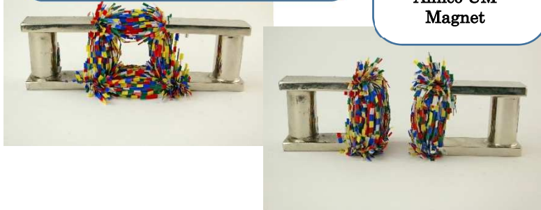
Using two magnets to realize two magnetic forces (attractive and repulsive forces)
