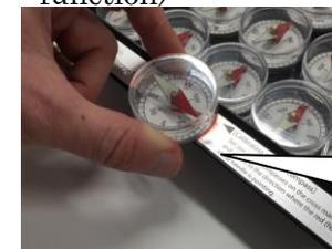
A compass on calibration area of which needle is pointing the right.
