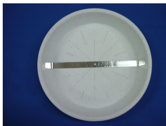
Photo 4. Attaching the Electrodes according to the Marking (Wipe the bottom of the tray with tissue paper dampened with alcohol before attaching the tape.)
