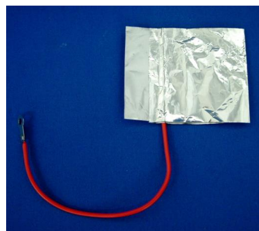
Attach the aluminum tape with the lead to the aluminum foil (electrode).
