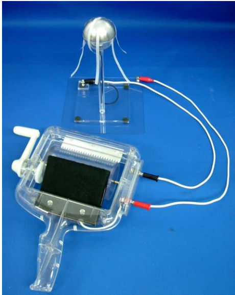
Photo 2. Connection with the Electrostatic Generator
