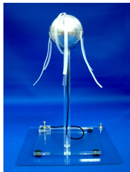
Photo 1. Aluminum Collecting Sphere with Paper Strips Attached
