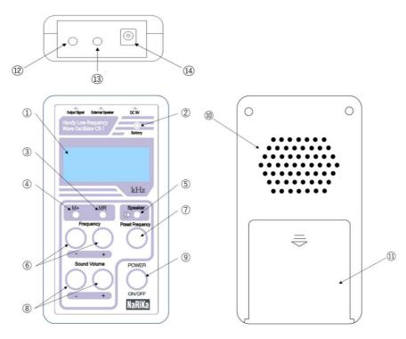
① Display Screen Display the current frequency (in kHz).
