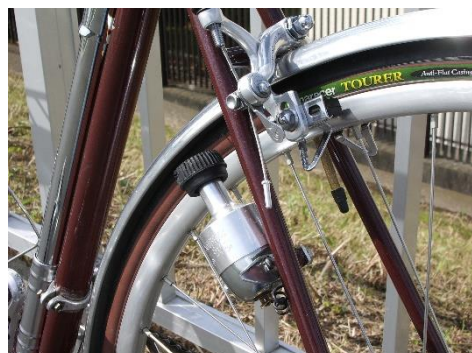
Bicycle with typical dynamo attached (small generator)
